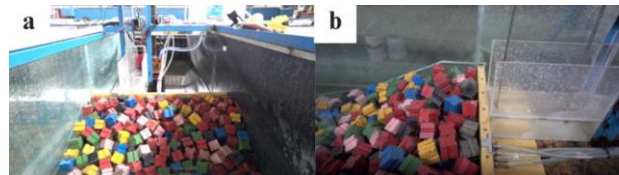
Figure 2 - A close view of the cross-section in the wave flume (a) front view, (b) side view. (In this figure, the irregular placement of the Antifer units is shown.)
