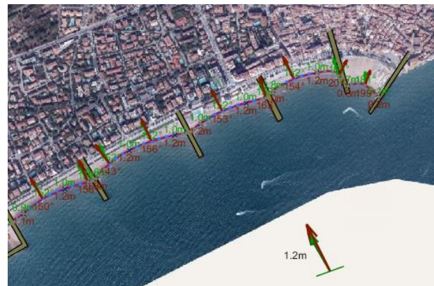
Figure 7 - Bypassing at revetments
