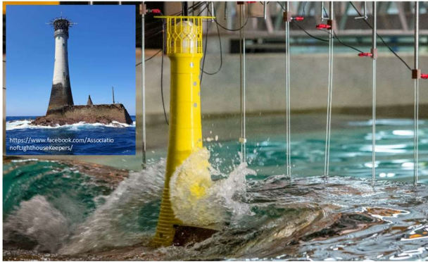
Figure 3 - Model Tests in the Ocean Basin, Plymouth, UK
