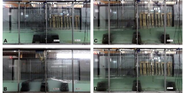
Figure 1 - Photographs of wave interactions with different layouts of the modules tested with no spacing between rows (A) through to a spacing of three module diameters between rows (D).
