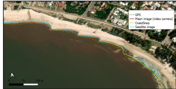
Figure 3 - Comparison of video, CoastSnap and Satellite derived shorelines, with in situ measured shoreline (GPS), for Atlántida, Canelones.
