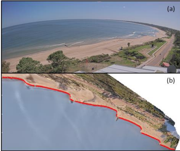
Figure 2 - Example of a camera frame (a), and orthorectification and shoreline detection (b).
