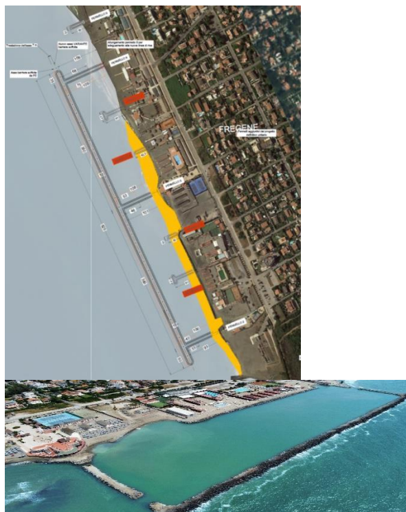
Figure 3 - Plan of the new protection works at Fregene, with drone view of the ongoing works in 2023.
