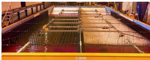
Figure 1 - Experimental set-up. Mangrove mimics at the left side and saltmarsh mimics at the right side. The smooth rigid slope covered with white vinyl is at the end of the wave tank and pink water can be observed due to the use of rhodamine for dyeing.
