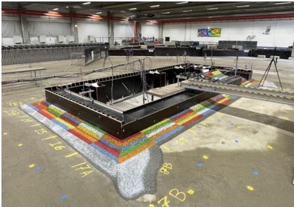
Figure 2 – Model and bathymetry constructed in 3D (DHI)
