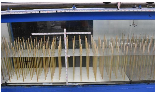
Figure 1 - Artificial vegetation and sediment bed during the experiments in the wave-current flume at MIT.
