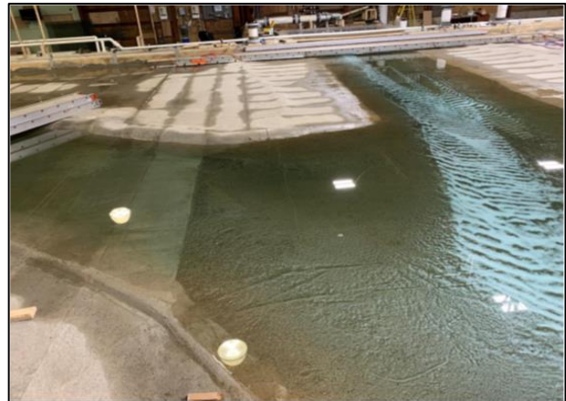
Figure 4 - Sediment Tracer in Physical Model (Looking Downstream of Brazos River)
