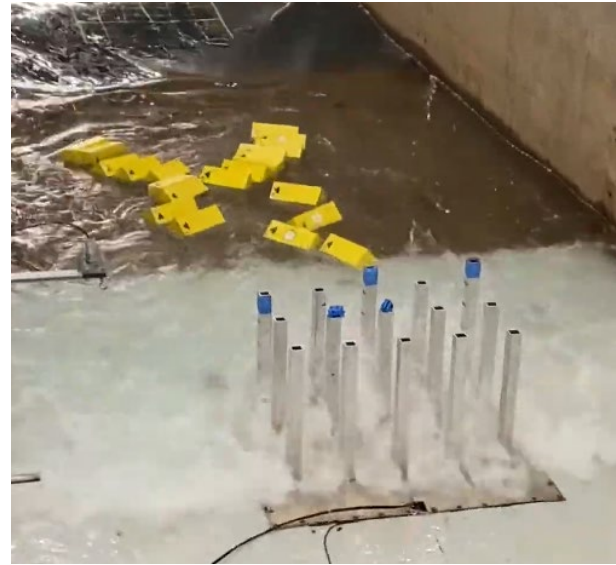
Figure 2 - Image of waterborne debris transported by a tsunami-like wave prior of impacting a set of vertical columns. Impact and damming loads were measured at selected individual columns and overall forces were measured for the whole specimen.
