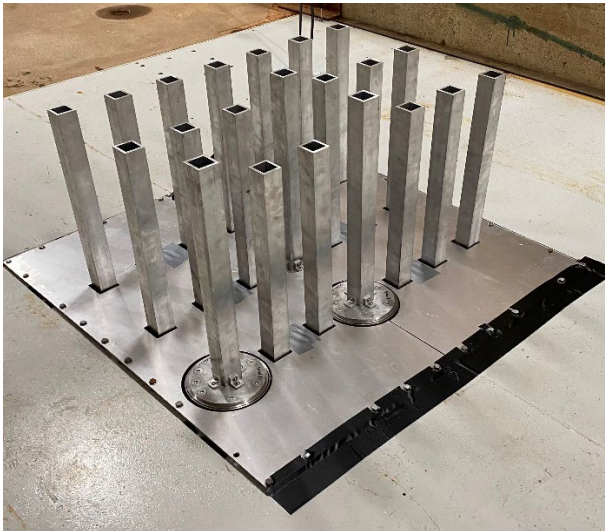
Figure 1 - Design render and constructed model of the complete set of vertical slender columns during the tsunami debris damming experiments.
