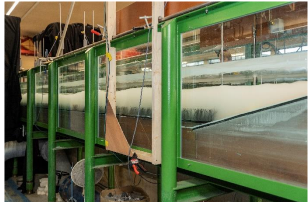
Figure 1 - Side view of the wave flume, at the toe of the dike.
