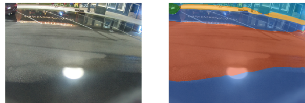
Figure 1 - (A) Image of roadway flooding during inundation of stormwater network in Beaufort, North Carolina, USA; (B) predicted segmentation from ML algorithm showing water (dark blue), roadway (red), sidewalk (orange), vehicle (green) and building (light blue).
