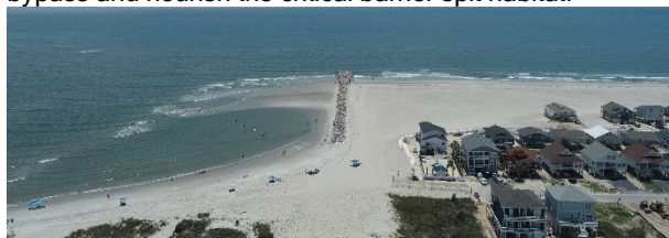
Figure 3. Post-construction drone image of the preferred alternative showing a prominent bypassing bar developing immediately after construction of the project.
