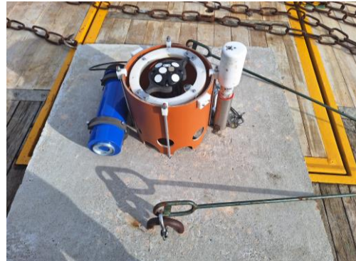
Figure 1 - Bottom mounted ADCP before deployment
