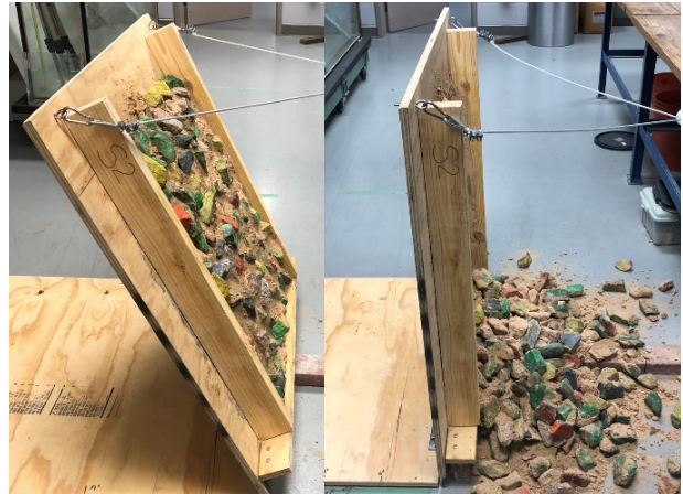
Figure 2 - Rock revetment slope test with MICP enhanced sediment before (left) and after failure (right).
