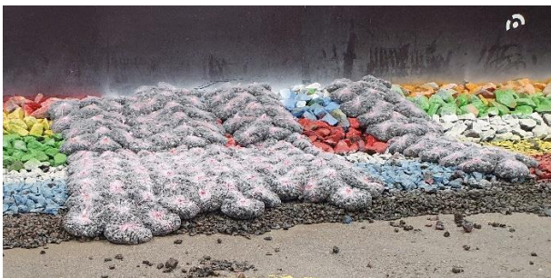
Figure 2: Rock bags installed over a scaled cable for 3D physical model testing at DHI
