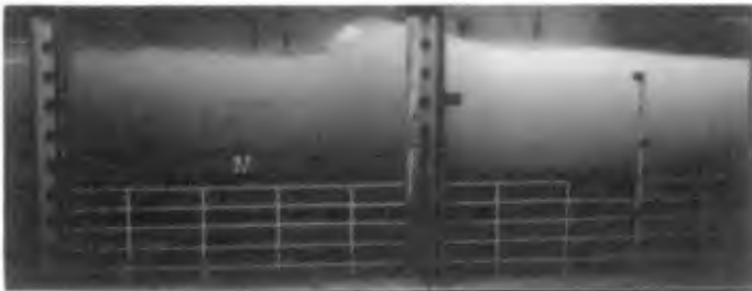
Photo 1 Effect of progressive waves on a loose sandbed.
