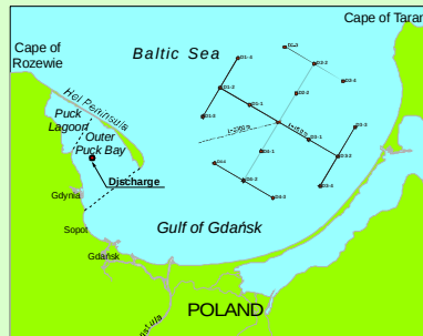
Study area with chosen location of discharge and scheme of diffusing system designed by EMPORIUM
