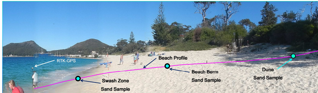
Figure 2 Field data collected on a NSW beach of Shoal Bay: i) profiles of beach-dune transect lines at 50m intervals, (2) three sediment samples at the swash zone, dry beach and dune face on the first transit, (3) dune toe elevations between the transects, (4) maximum wave runup levels of debris, and (5) site photos.
