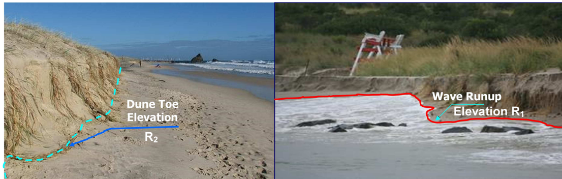
Figure 11. The conceptual model for assessment of beach-dune erosion: It states that a beach-dune system with R_2 < R_1 is expected to keep moving landward until such a time when the condition of R_2 > R_1 is reached.
