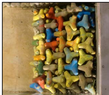
Figure 12. Result of Tetrapod (28.8 t) after 7.1 m overflow
