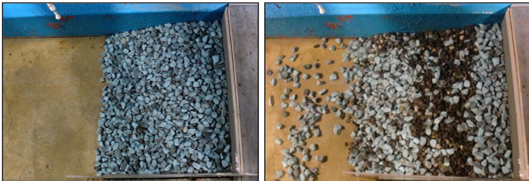
Figure 8. Damage to the 1.0 t armor stones (left: before overflow, right: after 7.1 m overflow)
