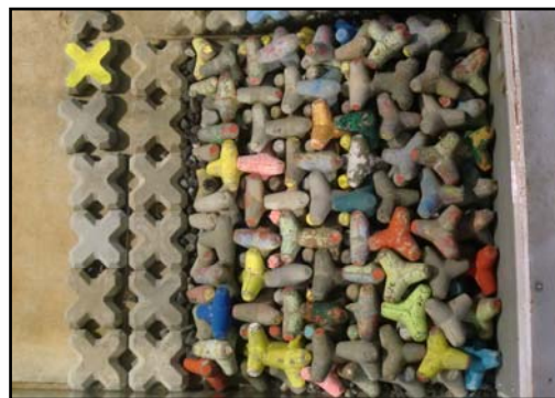
Figure 14. Result of Tetrapod (14.5 t) reinforced by placing X-Block (30.5 t) after 7.1 m overflow
