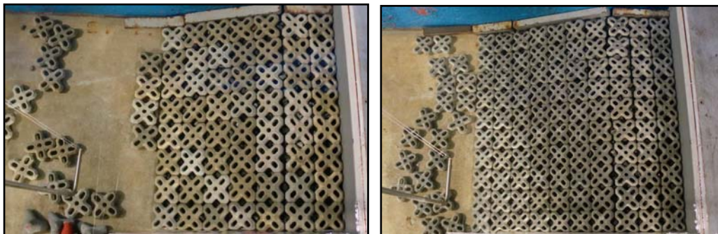
Figure 11. Damage to Permex after 7.1 m overflow (left: 8.1 t, right: 4.1 t)
