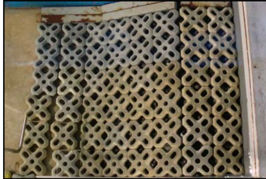
Figure 10. Result of Permex (16.1 t) after 7.1 m overflow
