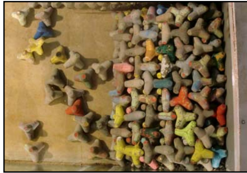
Figure 13. Damage to Tetrapod (14.5 t) after 7.1 m overflow
