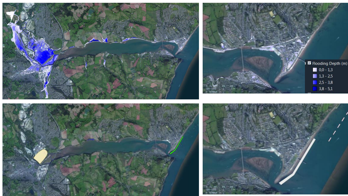
Figure 5. Flooding Depth: No mitigation options (up) vs All mitigations (down). Close up of detailed maps (right panels), for Mid-term conditions: 2050 yr, Tr 50 yrs.
