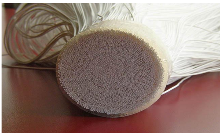
Figure 4. Hollow fiber membrane module in a submerged MBR system
