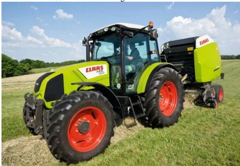
Fig. 2. Axos 340S tractor with a semi-trailer for fodder harvesting machine
