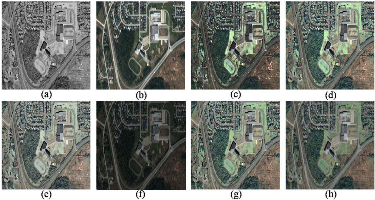
Fig. 8. Fusion Results of IKONOS-2 image (a) 1m Panchromatic image (b) 4m Multispectral image (c) IHS Method (d) Modified IHS Method (e) PCA based method (f) WT based method (g) Brovey Transform Method (h) Proposed Method
