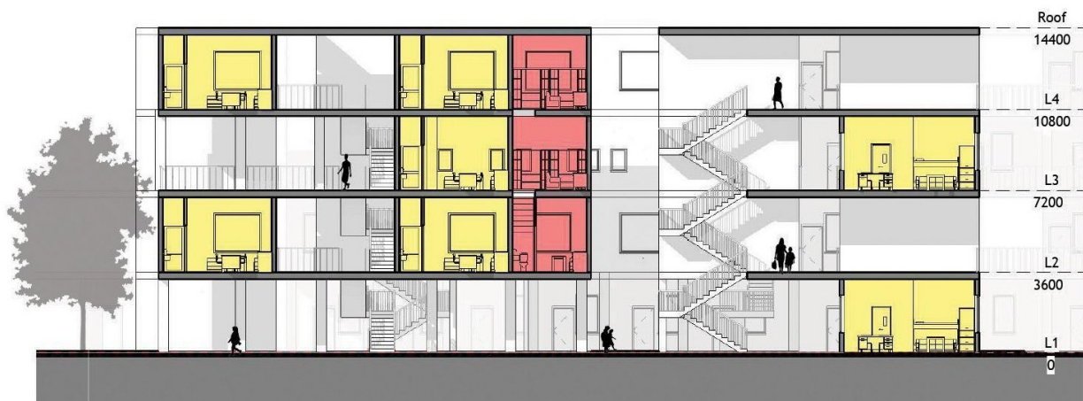
Figure 8. Section showing alternating vertical open spaces of Toan Le Phuc's project.
