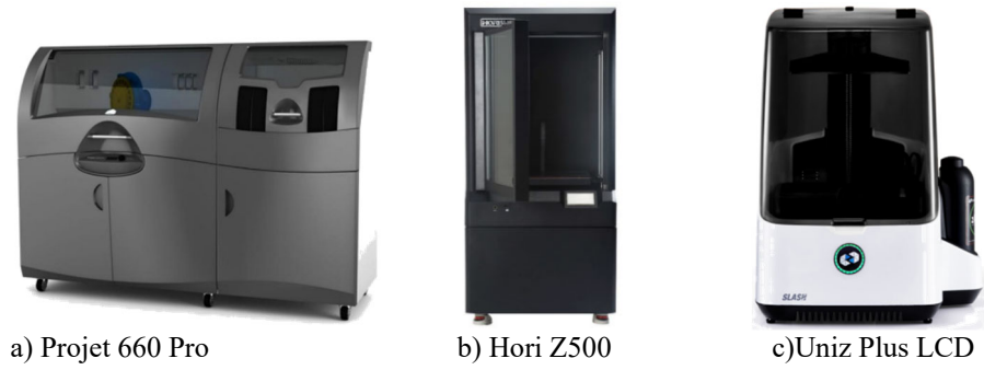
Figure 3. 3D printing equipment
