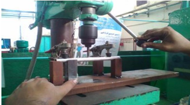
Figure 14. Initial fixture layout for Al-T3 pipe
