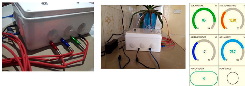
Fig. 5. IoT sensor setup: (a) Sensors, (b) Complete setup, (c) Real-time readings
