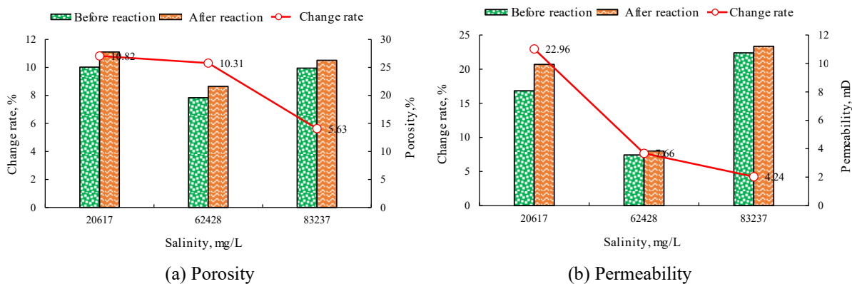
Figure 7. Changes in porosity and permeability before and after reactions at different salinity.
