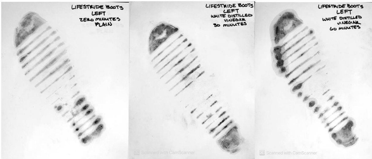
Fig. 3. Shoe print results of Lifeslide women's left boot without white distilled vinegar and with white distilled vinegar after thirty and sixty minutes.
