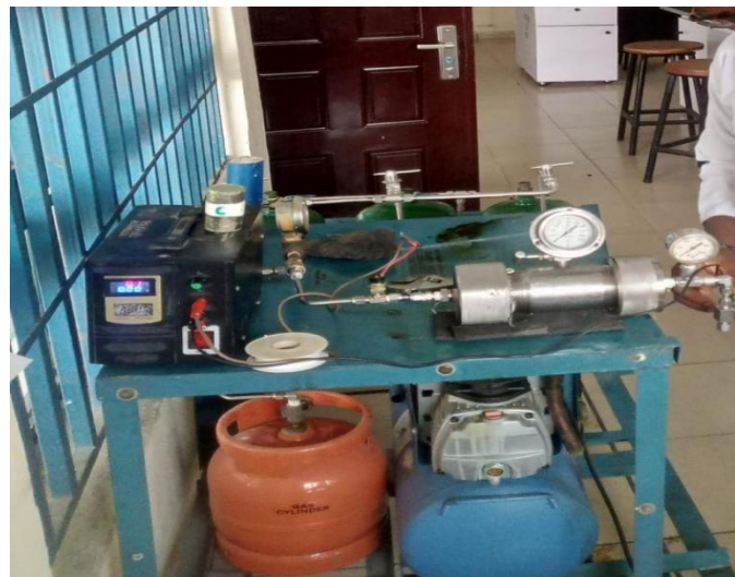
Figure 2—A schematics setup of an electrokinetic core flooding equipment (FUPRE LAB).
