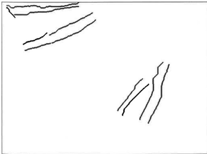
Fig. 2: Processing steps of R-SEED detection: (A) binary image resulting from one specific threshold, which is optimal for the upper left region, (B) all regions selected as R-SEEDS using a set of varying thresholds: borders from thresholding and pixel pairs to be connected by the A*-algorithm, (C) final R-SEEDS resulting from A*-connection. These are the R-SEEDS shown in Fig. 1 using a different representation
