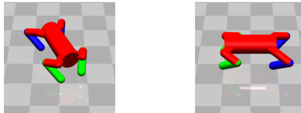
Fig. 17. doggo robot: a quadrupedal robot with bilateral symmetry with 12-dimensional control space.
