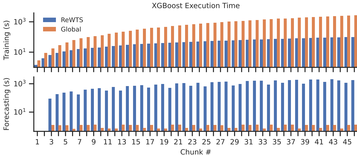
Fig. 13. Comparison of training and forecasting execution times for the global and ReWTS ensemble methods on wastewater treatment plant data using the XGBoost model (logarithmic scale).
