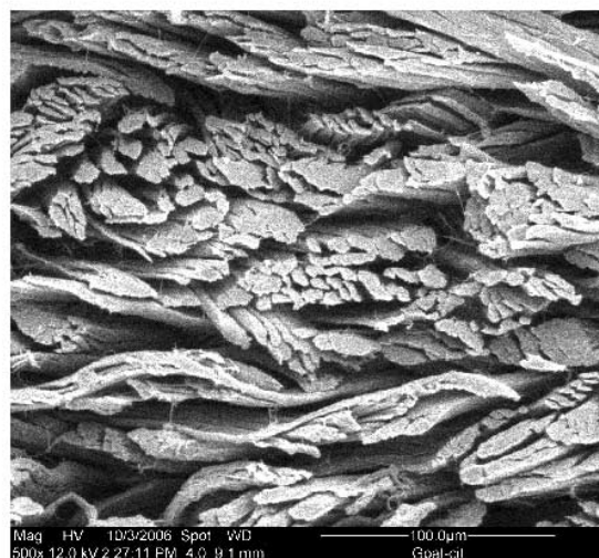
Figure 9: Scanning electron microphotograph of iron- citrate tanned goat suede leather showing the cross section at 500x
