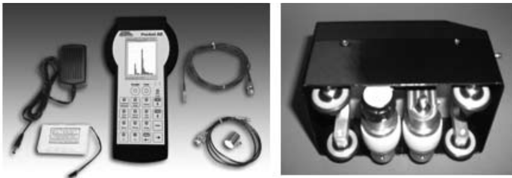
Figure 10: A newly designed portable AE system for the evaluation of leather quality: (a) Pocket AE-1 system proposed to be the system platform, (b) Prototype rolling sensor to be used in leather evaluation.
