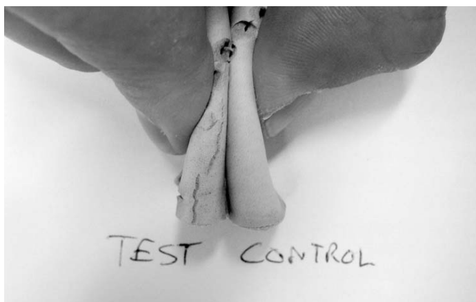
Figure 9. Air dried wetblue showing grain rupture on the test (molded leather) and intact control
