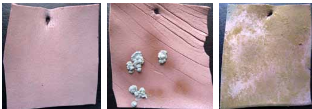
Figure 6: Crust leathers with 0.1% Azole 388 (left), 0.1% TCMTB 30 (center) and no fungicide (right) after 4 weeks of tropical chamber mold resistance testing. The crust leather on the left has no mold growth (mold rating of 0), which indicates the leather possesses long-term mold resistance. The leather in the center has a very moderate degree of mold growth (mold growth rating of 15). The leather on the right is fully covered with mold growth (mold growth rating of 100).
