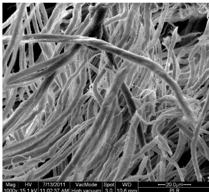
Figure 3: Scanning electron microscopic photograph [x 1000 magnification] of grain surface of the leather fatliquored using FL R, containing conventional sulfonated surfactant
