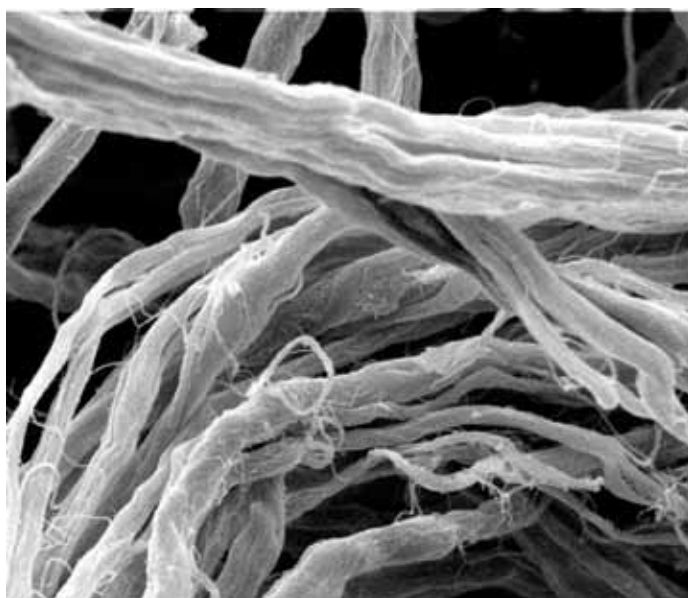
Figure 7. SEM photograph of resultant leather treated with fatliquor FL2 prepared out of amphoteric surfactant DEALI at a magnification of X 2000
