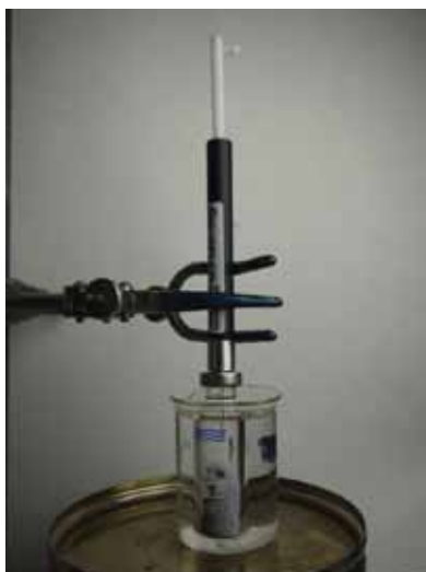
Figure 3. Image of HS-SPME extraction process.
