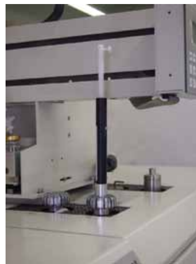
Figure 5. Image of HS-SPME desorption process in the GC injector.
