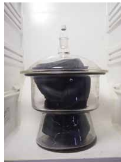
Figure 6. An adapted desiccator placed in an oven was used as an extraction chamber for the HS-SPME method.
