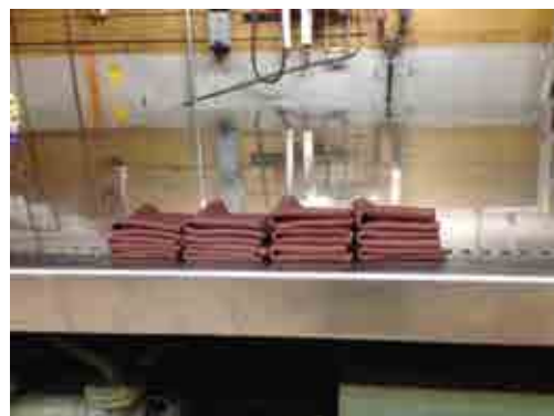
Figure 4. Wet white hides that had been treated with a 6% offer of gelatin (based on wet weight of hides and carried out in a 300% float) and then were retanned colored and fatliquored. Six pieces on left are untreated control samples, six on right had been treated with product.
