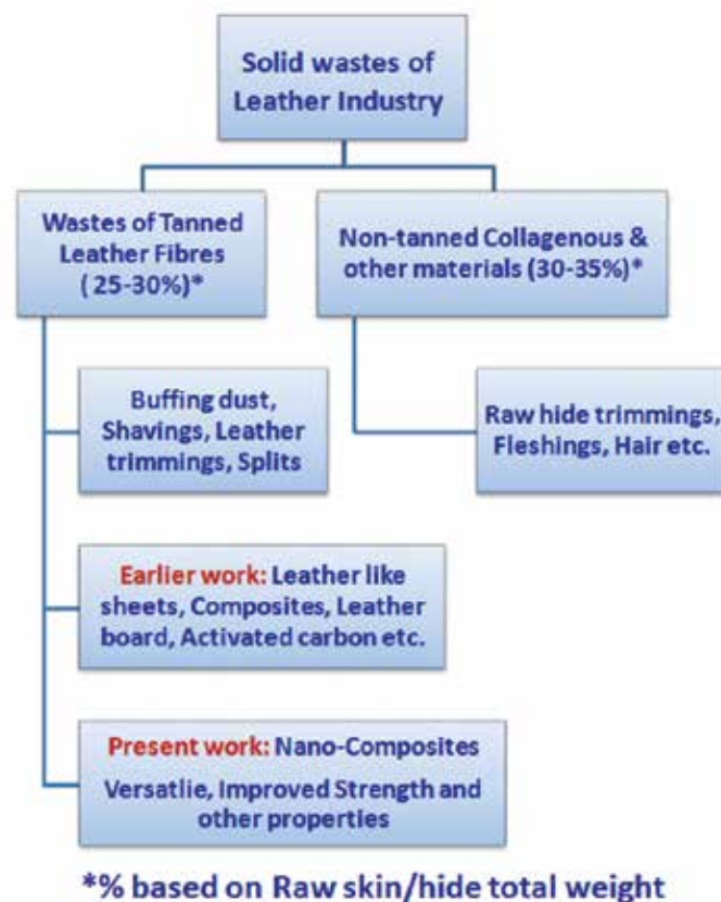
Figure. 1. Scope of the present work: Different solid wastes generated in leather processing and their possible utilization.
