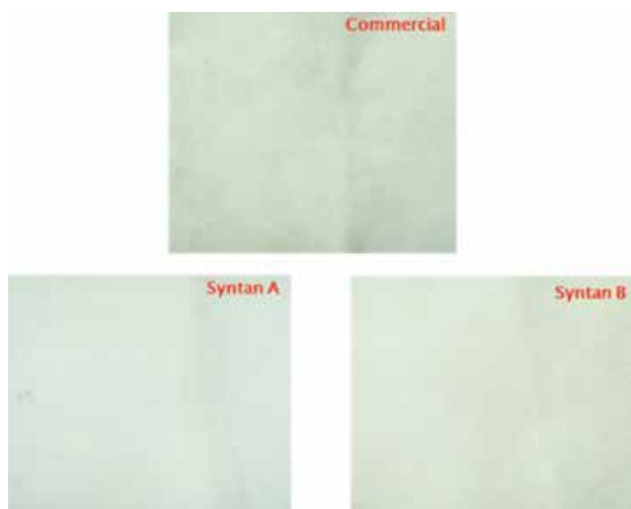
Figure 5. Color of the crust leathers made from commercial phenolic syntan and experimental Syntan A and Syntan B.
