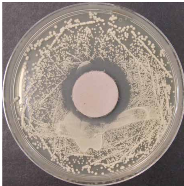
Figure 2. Leather fatliquored with thyme oil, view from the grain side - growth inhibition zone for the yeast Candida albicans (after 6-month storage).
