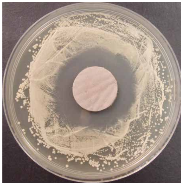
Figure 3. Leather fatliquored with cinnamon oil, view from the grain side - growth inhibition zone for the yeast Candida albicans (after 6-month storage).
