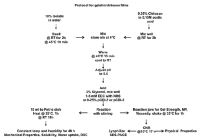
Figure 1. Flow diagram for preparation of carbodiimide-modified gelatin and gelatin/chitosan biopolymer materials and films.
