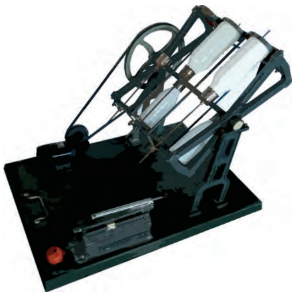
Figure 2. Photo of custom-made laboratory equipment used for washing and soaking of horsehide samples.
