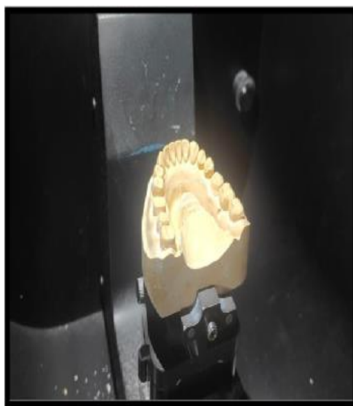
Fig5 Scanning of cast with desktop scanner
