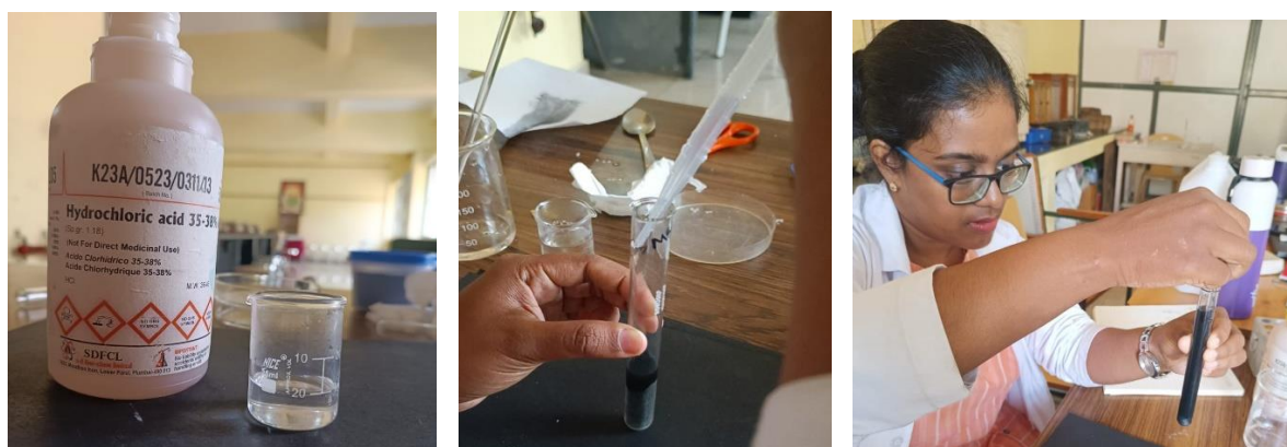
Fig. 26: Preparation of solution of sample with 20% Hcl
