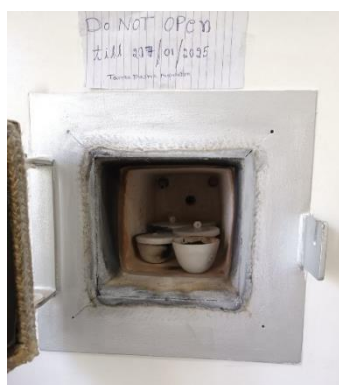
Fig. 14 & 15 Crucibles placed in the muffle furnace
