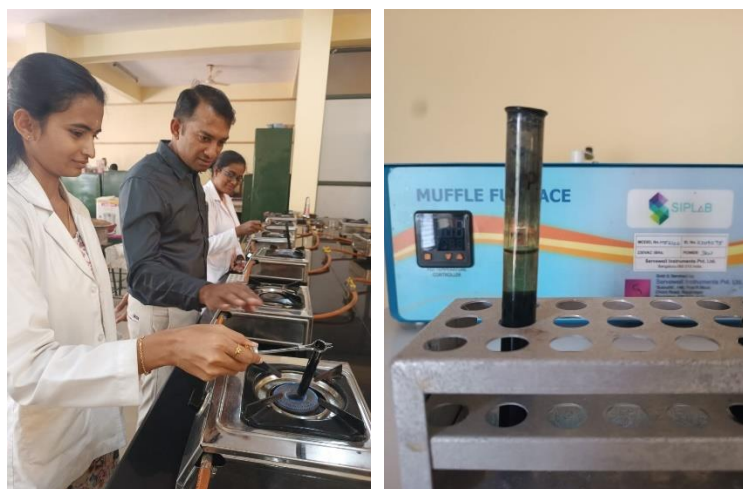
Fig 27: Heating the sample Fig 28: Supernatant part
